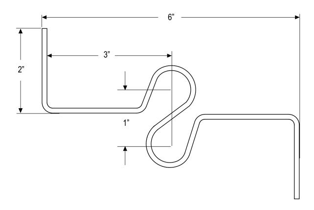
Wire (Carbon Steel): Prefabricated from cold-drawn steel wire conforming to ASTM A1064/A1064M
