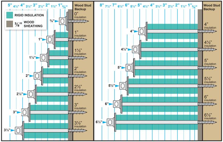
Concrete Seal Tie™ is an innovative single screw veneer tie suitable for use with concrete, CMU, wood stud, or brick backup.
